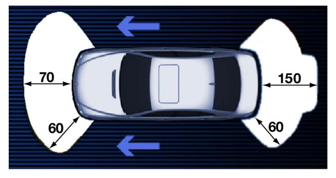
The closer the vehicle comes to the object, the shorter the frequency of the signal becomes. If the distance to a detected object is smaller than approximately 30 cm (11 in.), a continuous tone is issued.
